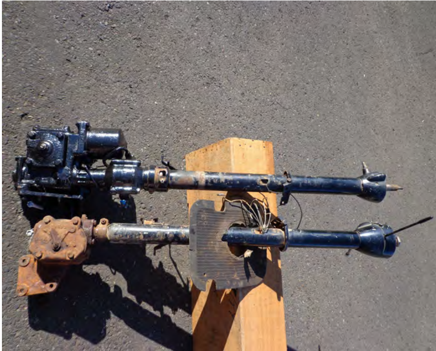
Comparison of the two steering columns. The top one shows the column with the power steering gear. The bottom one shows the column with the standard gear. Photo courtesy of Brent Hagen
