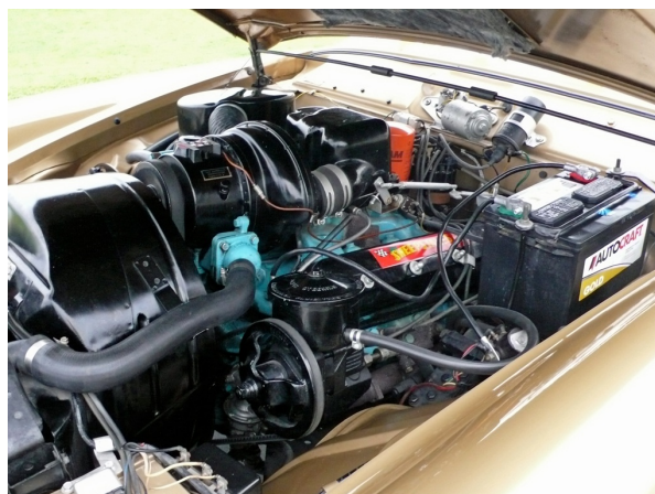
The supercharged V8 for 1957 Golden Hawks Photo courtesy of owner Barry Maxwell
