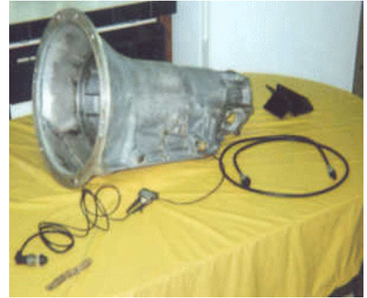
Shift linkage arm (rod not pictured)
