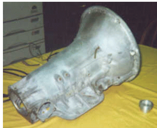
Torque converter to crank adapter bushing
