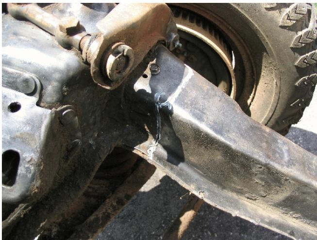
I thought I would mention to you, while cleaning the front frame, I noticed a substantial crack on the right member about 2-3" back from the front crossmember. It is not because of any rust as there isn't any, wondering if this is a common problem? It starts at the bottom of the right rail, goes up and across the top, where it stops. It is an easy welding repair, now the engine is out.
