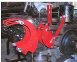
**Do You Want dependable air conditioning** for your 1955-56 V-8 Packard engine in whichever car it is in? You will need the third puller and bolt for the crankshaft to drive the compressor. Modern, dependable serviceable equipment starts with the Sanden
