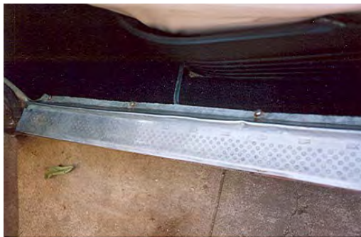
The best of the three photos clearly shows the carpet under the scuff plate
