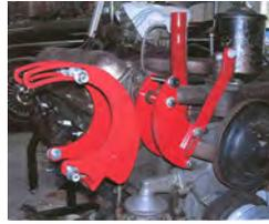
**Air conditioning** for 1955-56 V-8 Packard engine in whichever car it is in. You will need the third pulley and bolt for the crankshaft to drive the compressor. Modern, dependable, serviceable equipment starts with the Sanden
