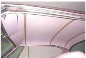
In 1998, the headliner perforated cardboard started to separate from the fiberglass backing that Phantom was using at the time. I called Rene Harger at Phantom and he graciously replaced all the headliner pieces, saying that it
