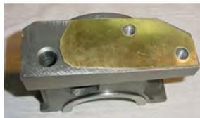
A pump-to-adapter gasket was made from 0.010in brass shim stock. This version does not have the center oil passage hole because of the companion full-flow oil filter conversion. Brass was used to make the gasket because there is a slight overlap between the discharge hole in the Olds oil pump and the two counter-sunk holes ("P" above).
