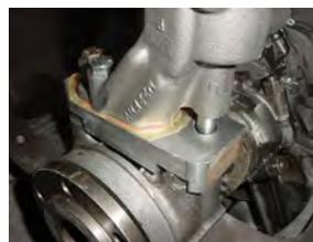
The Olds High Volume oil pump adaption bolted to Kevin's engine.
