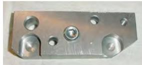
This side of the adapter mates to the rear main cap. The 3/8NPT plug in the center is for the companion full-flow oil filter conversion only. It seals the hole which connects the pump to the oil gallery in the rear main cap. If only the Olds pump is to be fitted (no full-flow conversion), then this hole will be open.
