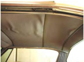
In 2007, I noticed that the cardboard was starting to bubble away from the backing again and it only got worse in damp weather. See photo #3 for the extent of the damage. I contacted the new owners of Phantom about the recurring
