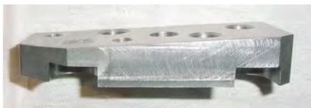
Rear view of the adapter. The reliefs on the bottom are to clear the stock rear main cap bolts. The adapter is machined from mild steel. NOTE the 5-degree angle of the pump mating surface.
