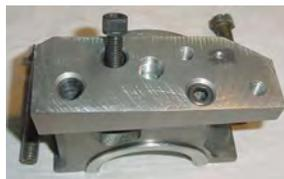
This shows the allen-head cap screws used to attach the adapter to the rear main cap. The holes are countersunk so they will not interfere with the Olds pump mounting face.
