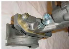
The Olds High Volume oil pump is attached to the adapter with brass gasket in place. The AN-10x3/8NPT fitting in the side of the pump is for the companion full-flow conversion only.
