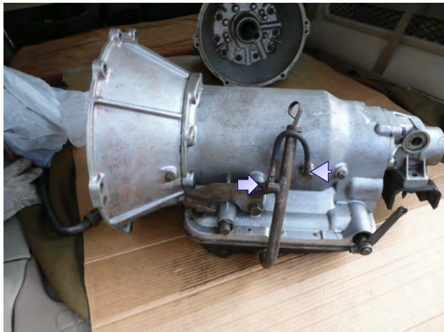
A fitting is attached to the filler tube, with a hose running from it to the vent. Photo by Gus Daub
