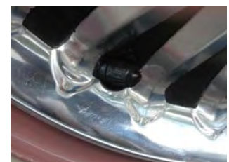
Front tire, close-up of cocked stem
