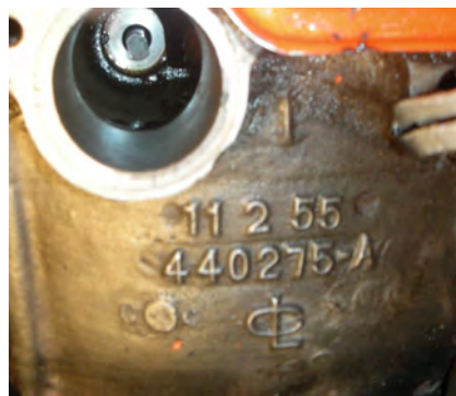
This photo shows the casting number on top of the flywheel which further proves I've got a 1955 Clipper Custom service replacement engine.
