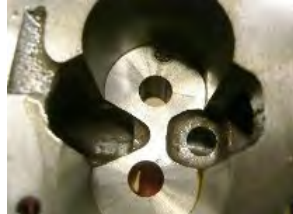
output side of new pump (6492430)
