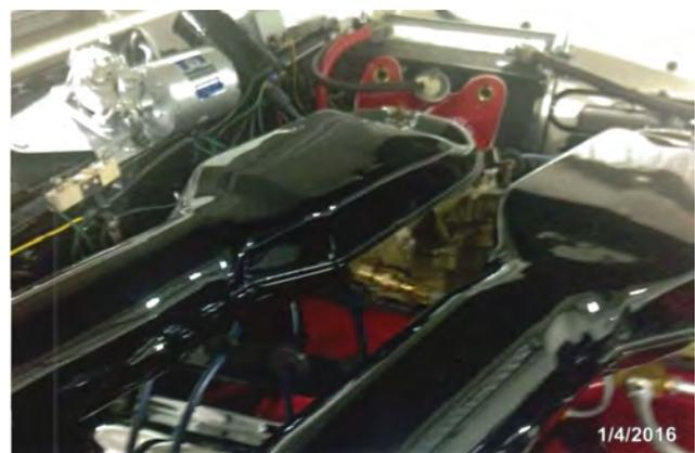
“The air cleaner at the bottom appear to be a standard type. There is no support bracket from the engine to the bottom of the air cleaner.”
