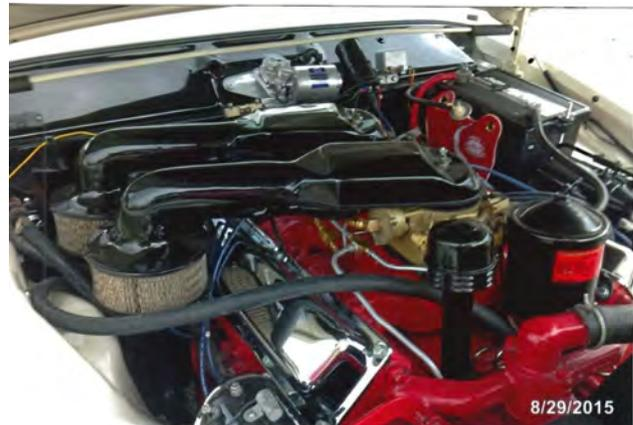
“The part that attaches to the carburetor appears to be the same as the standard oil bath, but once the narrow area is reached, the material is aluminum and is only about 3-4 inches in diameter.”
