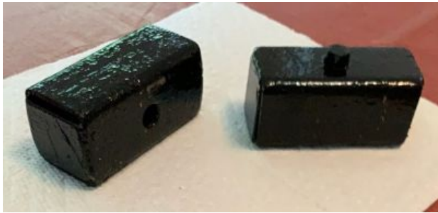
These are homemade 2" lowering blocks... I will install them in my '56J, as I'm using 1957 Stude station wagon leaf springs, which make the Hawk sit too high at the rear for my liking.
