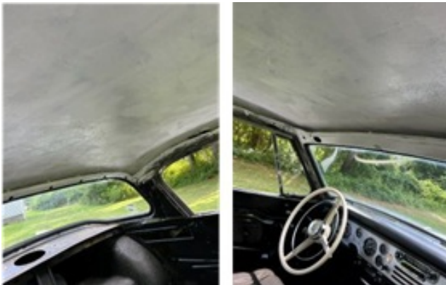
Underside of roof scraped, wire brushed, and covered with a coat of SEM 'rust converter' white paint. If I can accomplish the new windlace install, and then the multi section headliner, the rest will be easy peasy!
