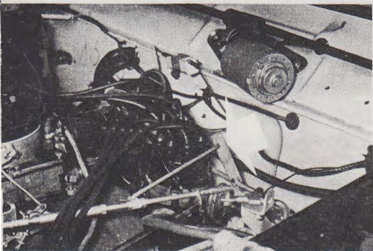
Arrow points to bellcrank arm that connects throttle linkage to transmission. Holes in arm adjust transmission shift points.
